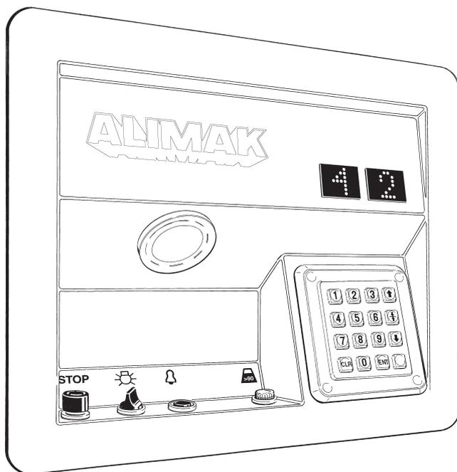
Keypad panel inside the car appl. for construction hoists
